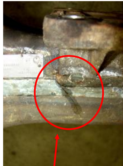
Cracked Axle Housing
