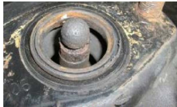
Corrosion on ball end of actuator and liner part of seal
